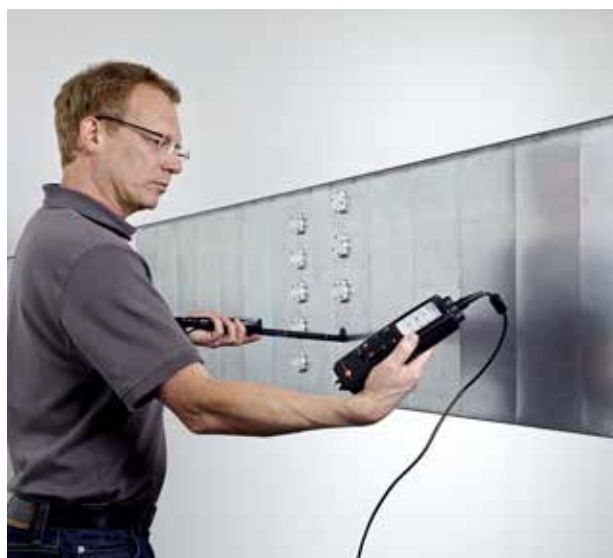
On-site volume flow calibration using an impeller pressure gauge in accordance with DIN EN 12599
