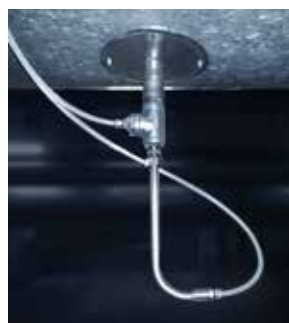
Fig. 3: Dynamic pressure probe for measuring the flow of the 300 °C air used for drying vehicle finishes.
