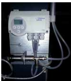
Fig. 4: The volume flow is recorded by the highly precise P26 differential pressure transmitter from halstrup-walcher
