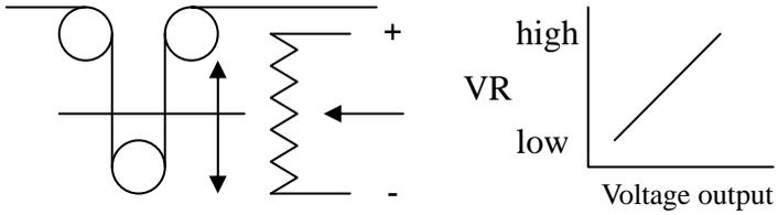
1. Set Pr09 at 3 and observe VR variations. Manually move VR wheel. The number has to be increasing between the lowest and highest points with the varying number of DC 4V at the least.
