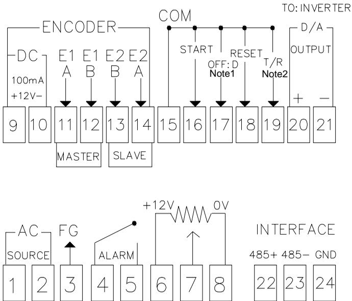
Note 1: When terminals 15 and 17 are short-circuited, 607 accepts VR input signal, but does not perform external diameter calculation. When they are open, 607 both accepts VR input signal and perform external diameter calculation.
