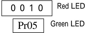
Then press **SET** to enter the change mode. Press **SET** after the change is made. Then press **MODE** to return to the operate mode.
