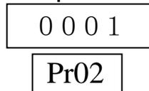
5. If Parameter 2 needs change, press SET to enter the change mode. Press  $\Delta$  or  $\nabla$  to select the function that needs change. Once the change is made, press SET to enter and the control panel switches to Parameter 3. Make a change to Parameter 3 in the same way as to Parameter 2.
