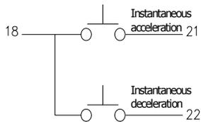
When Contacts 18 and 21 are connected, Slave can accelerate to 11m/min. The operator adjusts the speed until the cloth is no longer slack before releasing the differential push-button.
